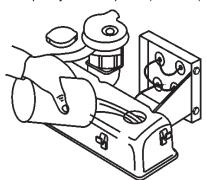
Figure 15. Engine Oil Filler Hole
